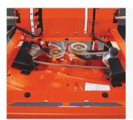
Removable foot pan Removable foot pan for easy access to deck belt pulleys, spindles and clean-up.
